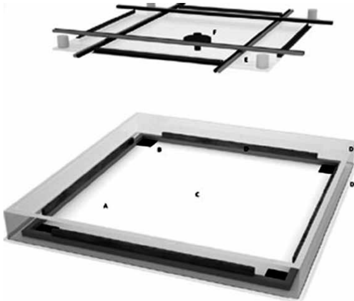
Figure 1. Three-dimensional rendering of the bed bug arena. (A) Area of movement. (B) Harborages. (C) CO 2 release point. (D) Safety barriers (polished plastic wall with copper weights, Plexiglas wall, insect glue-coated overhang, and mineral oil-filled duct). (E) White, red, and infrared light sources. (F) Vivotech IP camera.
