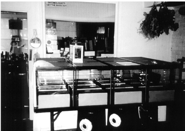
Figure 3. The use of 75-gallon aquaria as chambers for challenging the package resistance.
