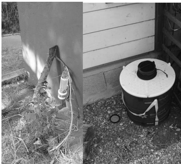
Figure 1. Mosquito sample collection with CDC Light trap (on the left) and BG-Sentinel (on the right).
