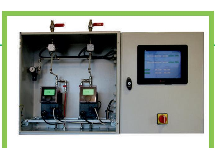
Part of the initial ULV spryer system prototype
