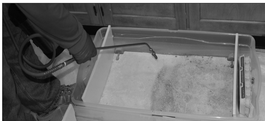
Figure 6. Chlorfenapyr spraying on concrete, wood or vinyl surface to the point of run-off with a B&G Sprayer equipped with flat-fan tip.
