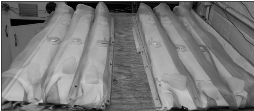
Figure 4. Experiment set up for wood and vinyl surfaces to delineate acute efficacy of chlorfenapyr against house flies. A 90 cm long x 12.5 cm wide strip was covered with 25 cm wide aluminum mesh to form a concave foraging arena.
