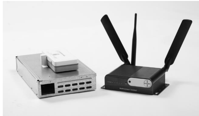
Figure 1, 2. Schematic illustrating the components in and operations of the Bayer Rodent Monitoring System . Images for a sensor and transceiver fitted to an industry standard multicatch mouse trap (L), and the LoRa gateway receives messages from the transceiver and routes them to the cloud database
